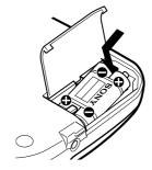
**3** Connect the AC power adaptor. The indication "CHG" lights up. Charge for about 2 hours (for BP-DM10) or 3.5 hours (for BP-DM20). (If the battery has been fully charged
